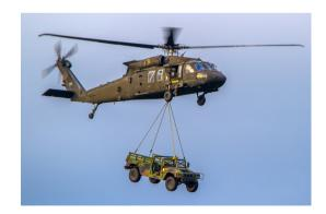
**Speed:** With two powerful General Electric engines giving it its strength, the Black Hawk possesses an amazing cruising speed of 174 miles per hour. It also has a rate of climb of 1,315 feet per minute, and a service ceiling of 19,000 feet.
